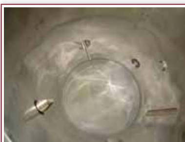
Figure 2. The novel design fluid bed NIR probe inserted into the product container of the fluid bed dryer. Note the collection "spoon" and purge vents.
