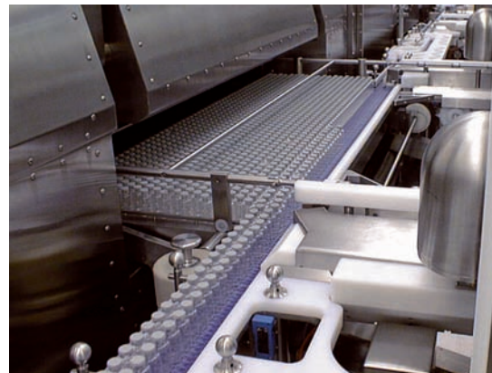
Conveyor-Pusher System in the isolator during charging
