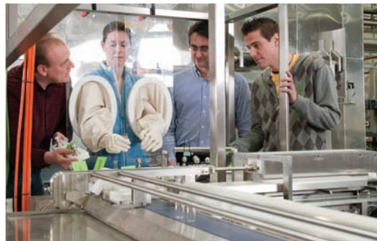
Mock-up is carried out with our customers so as to facilitate optimum ergonomics.
