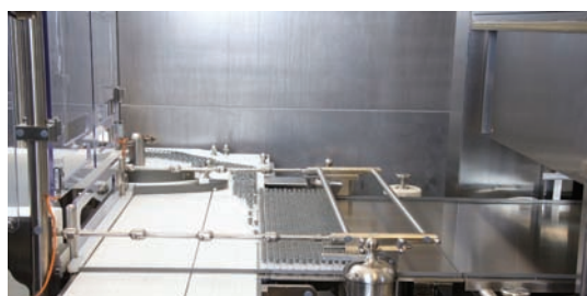
View of a Conveyor-Pusher System with RABS after freeze drying. The photos show the discharging sequence before the downstream capping machine.
