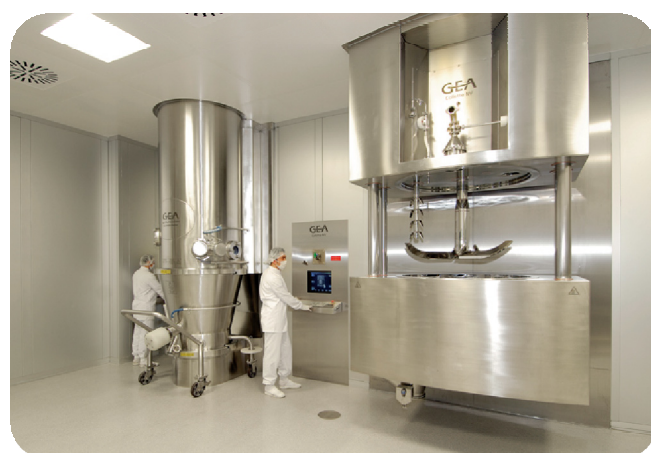
1. Integrated High Shear Granulation and Fluid Bed Drying Suite
