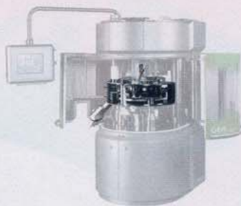
Figure 2 The ECM inside the tablet press.
