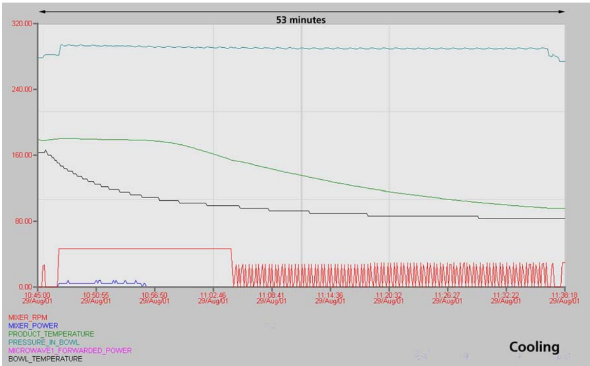
Figure 4b: graphical print-out of the cooling step using double jacket + pressurized air
