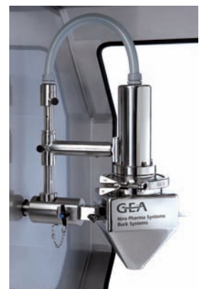
Measuring head and data analysing equipment discretely mounted onto the rotating blending head assembly.
