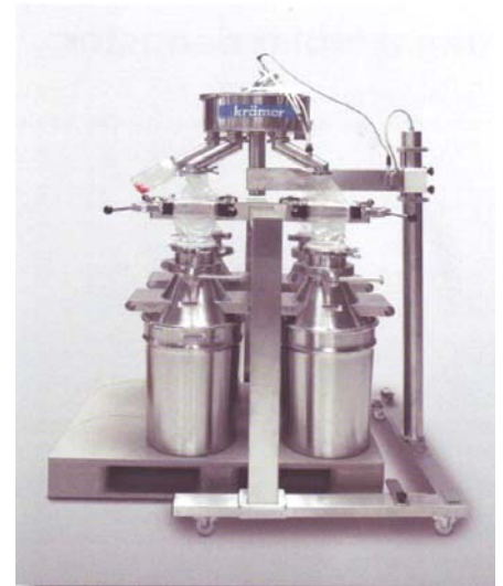
9. Hicoflex® container connection
