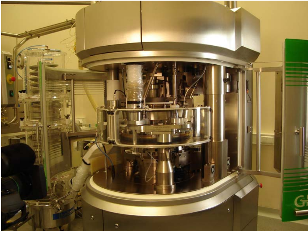
PHOTO 2: MODUL™ S with open front doors. WOL ECM visible
