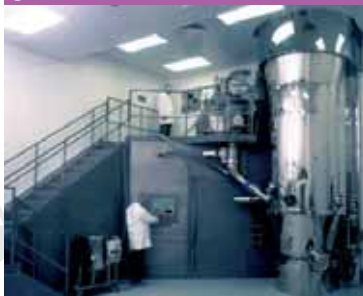
Figure 3 A typical set-up installation at an industrial scale for the production of pharmaceutical granules.
