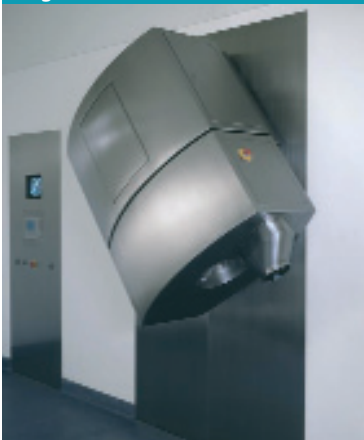
Figure 2 Single pot processor Ultima 75 (courtesy of Collette NV, Belgium).
